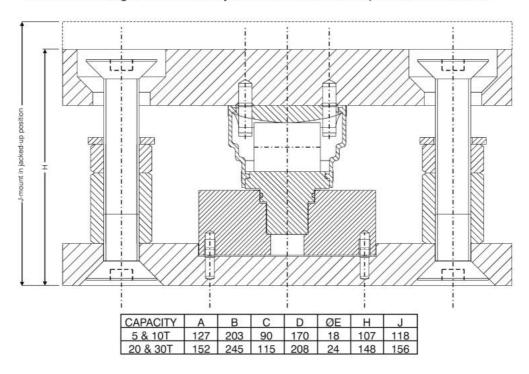
Mounting Hole Positions. All dimensions in mm.
