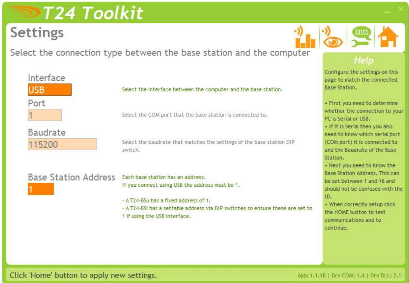
Select **USB** as the interface and select 1 as the Base Station Address. In the toolkit all items that can be changed by the user are coloured orange.
