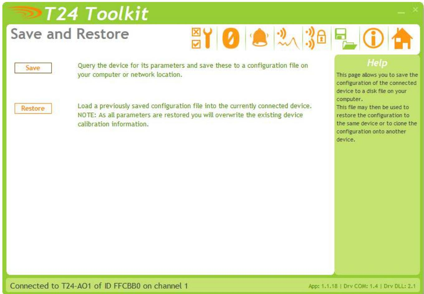
Here you can save the device settings to a file on your PC so that they can be later loaded back into the same or different device.
