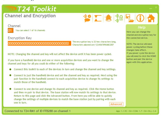
Here you can change the channel and encryption key for the module.
