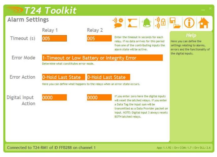
This page defines how the individual relays will react to time outs and errors present from any defined T24 device, as well as how Digital inputs 1 and 2 are used.
